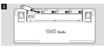
Insert four batteries (size AA) negative  $\bigcirc$  side first, then reattach the cover
