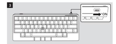
Turn on the power by sliding the power switch on the back of the keyboard to the right (it will turn green)
