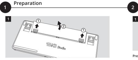
Slide the cover on the base of the keyboard in the direction of 1and lift it up in the direction of 2 to remove
