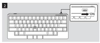
Turn on the power by sliding the power switch on the back of the keyboard to the right (it will turn green)
