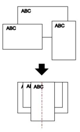
**2** Place the documents at the center of the ADF paper chute (feeder), and adjust the side guides to the widest document in the batch.
