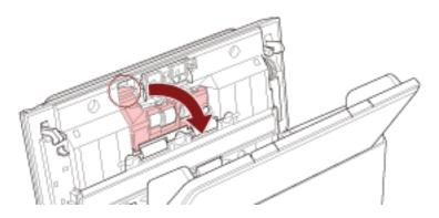
**b** Pull out the left side of the brake roller shaft, and then pull out the right side of the shaft from the hole.
