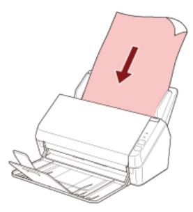
6 Adjust the side guides to the width of the Cleaning Paper.Move the side guides so that there is no space between the side guides and the Cleaning Paper.
