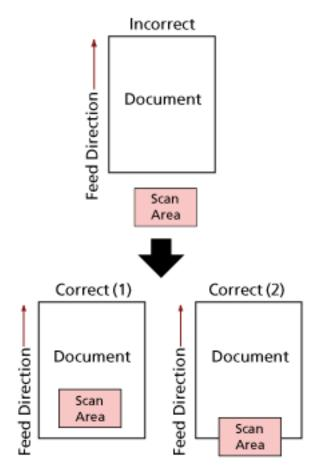
Outside of the document may have been scanned because the scanned document is shorter than the specified paper size.
