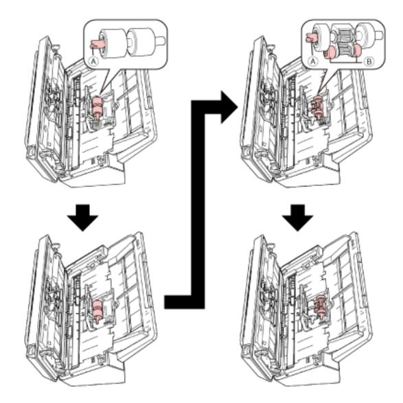
a Check the direction of the notch (A) on the pick roller and of the small roller (B), and insert it in the hole.
