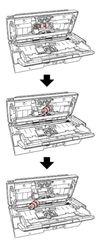
**4** Remove the brake roller from its shaft.
