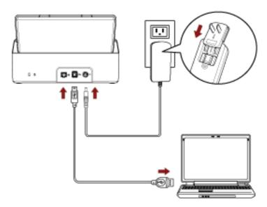
For details about how to turn on the scanner, refer to How to Turn the Power ON (page 30).
