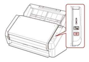
After the power indicator flashes for a while, the scanner is turned off and the power indicator switches off.
