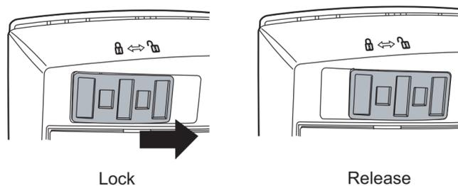
Make sure to slide the shipping lock in place (located on the bottom of the scanner) to secure the internal carrier unit during transportation. After transporting and placing the scanner, tilt the scanner (approx. 30 degrees) and release the shipping lock. See the "fi-4220C Image Scanner Operator's Guide" for further details.
