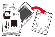
6 Remove the protection tape on the print cartridge.
