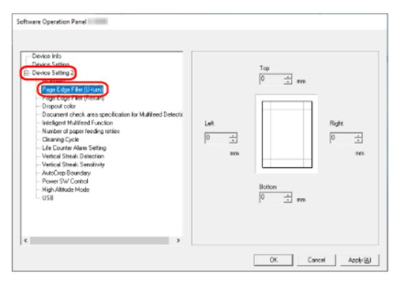
**3** Specify the width of each margin (Top/Bottom/Right/Left) to fill in. The factory default setting is "0". The specified area is filled in white or black, according to the background color.
