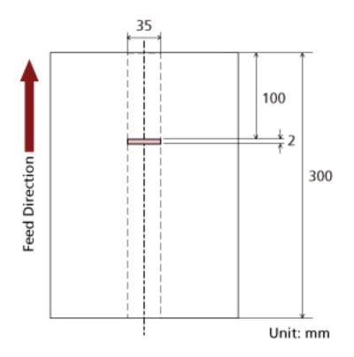
Since the detection area (length) is less than 5 mm, overlapped documents cannot be detected accurately.
