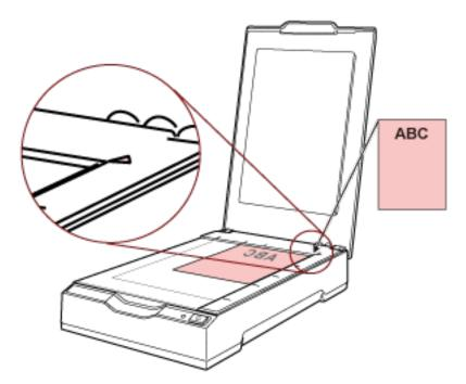
Place the document face-down to align its top left-hand corner with the reference point.
