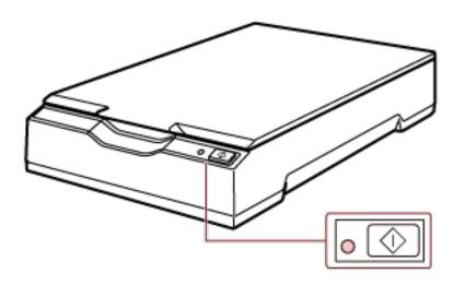
When the computer is turned off, the scanner is turned off and the power LED goes out.
