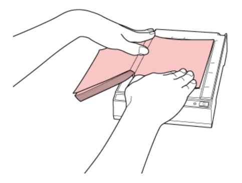
Place the document face-down to align its top left-hand corner with the reference point.
