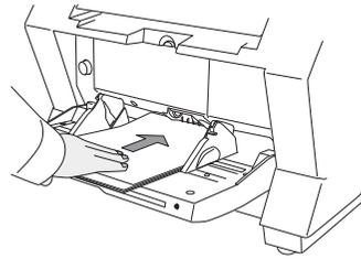
→ The document will be picked up, scanned and ejected into the stacker.
