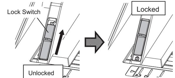
\* The load-bearing capacity of Lock Switch is limited. To slide the pair of Side Guides separately, secure one of the pair by hand while moving another.
