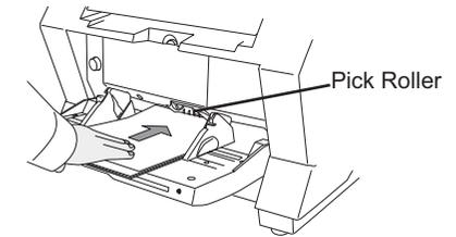
→ The document will be picked up, scanned and ejected into the stacker.
