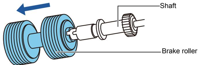
4. Attach a new brake roller on the shaft.
