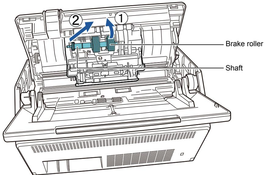
3. Remove the brake roller from its shaft.
