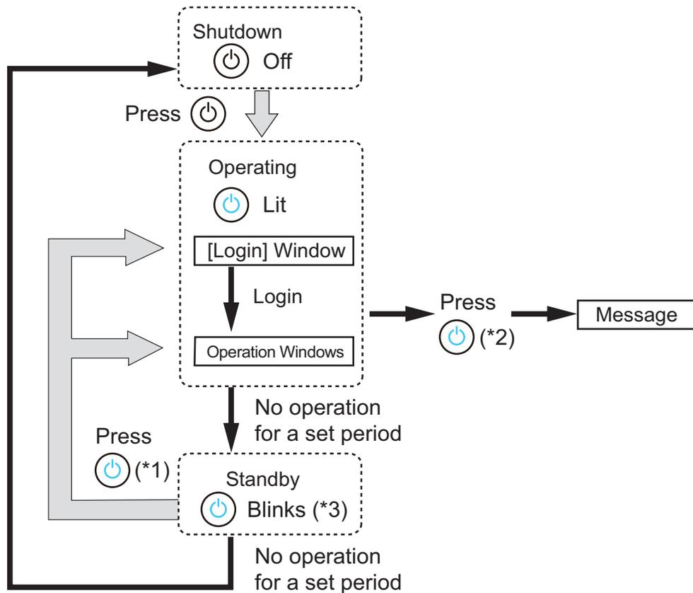
(\*1): The following operation will start up the scanner from standby mode.
