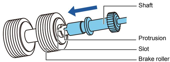
5. Install the brake roller with the shaft on the scanner.
