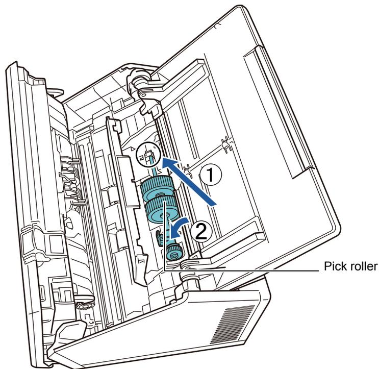
5. Rotate the lock release tab on the shaft in the direction of the arrow.
