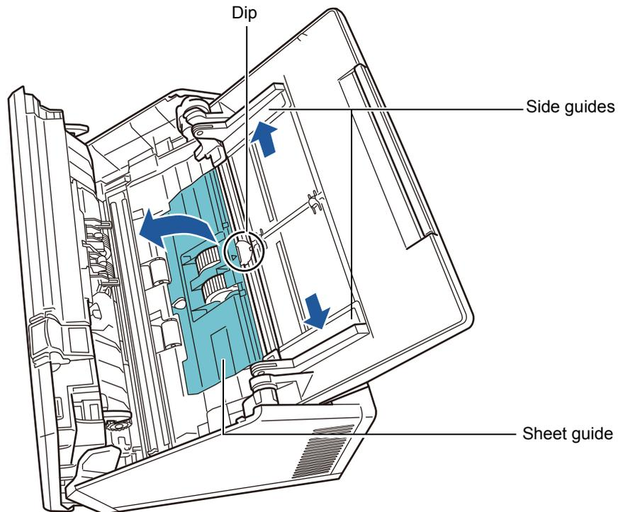
2. Rotate the lock release tab on the shaft in the direction of the arrow.
