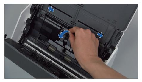
2. Rotate the bushing in the direction of the arrow.
