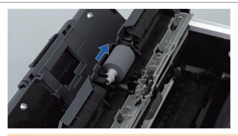
Make sure that the pick roller is attached firmly. Otherwise, paper jams or other feeding errors may occur.
