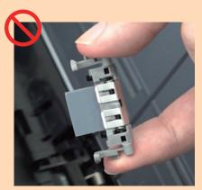
Make sure that the pad unit is attached firmly. Otherwise, paper jams or other feeding errors may occur.
