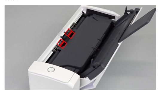
Gently wipe the dirt and dust off the rollers as you rotate them manually with a cloth moistened with Cleaner F1.
