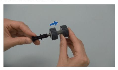
Attach the new brake roller to the shaft.
