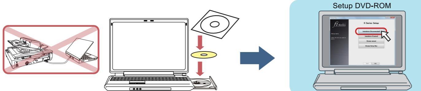
Be sure to install the required software before connecting the scanner to your computer.
