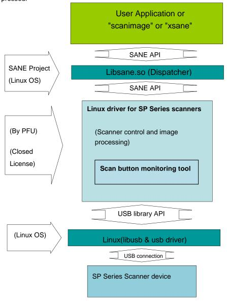
\*Note: In Linux systems, the term "driver" refers to a module that is installed in the Linux kernel and operates in privilege mode for the CPU. Previously, scanner drivers had been installed in the Linux kernel for operation. Currently, drivers are installed as a library based on SANE API outside the kernel and operate by dynamically linking from applications. Although it is actually a library, PFU and other scanner manufacturers call it a "driver".
